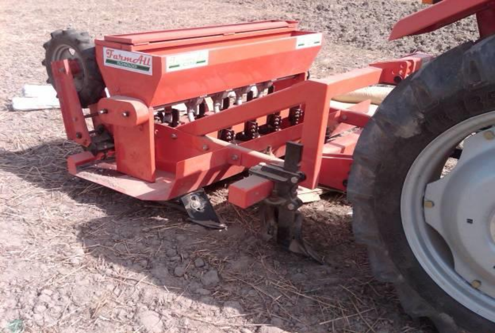
Mechanical transplanter for planting onto raised beds, made by machine
